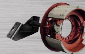
Wider brake lining for better brake response and higher life
